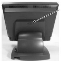
Press the Lock/Release button and lift the main unit to detach it from the paddle assembly.
